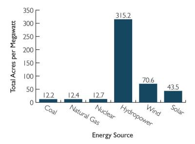
Coal, natural gas, and nuclear power all feature the smallest, and nearly identical physical footprint, of about 12 acres per megawatt produced. Solar and wind are much more land intensive technologies using 43.5 and 70.6 acres per megawatt, respectively. Hydroelectricity generated by large dams has a significantly larger footprint than any other generation technology using 315.2 acres per megawatt.
